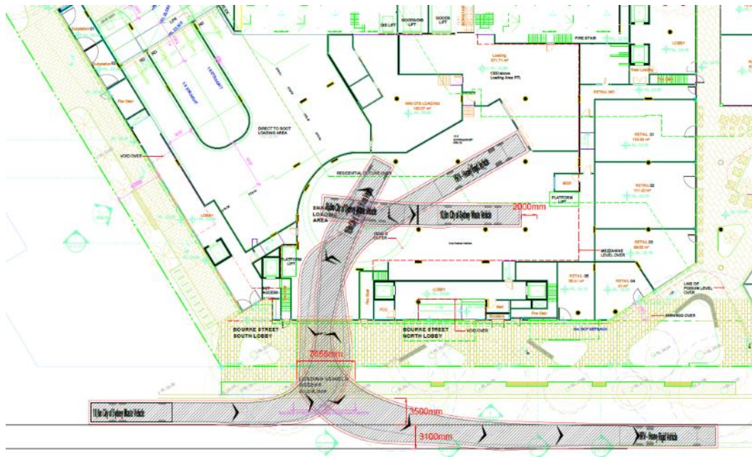
Figure 36: Swept path analysis for Heavy Rigid Vehicles
